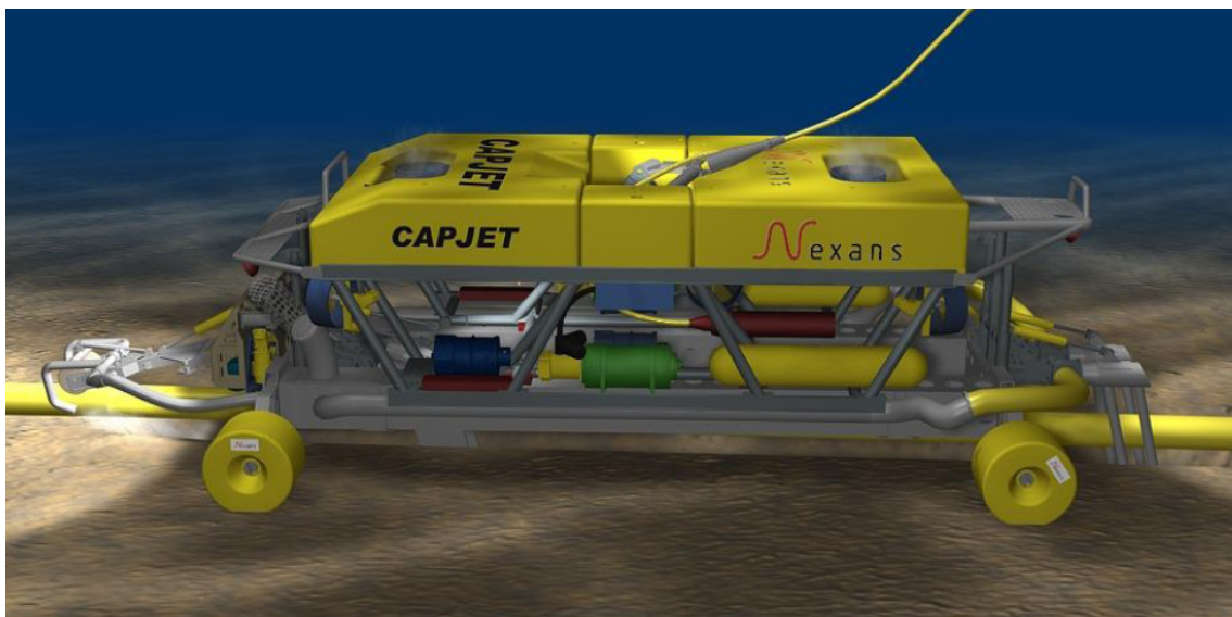
Figure 2.20 EXAMPLE OF JET TRENCHING MACHINE
